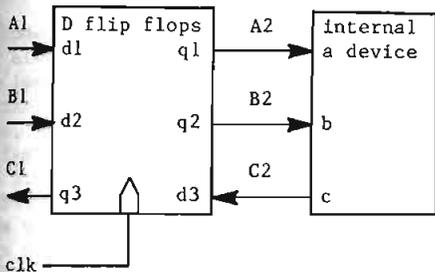
Figure 3: System Consisting of Flip Flops and an Internal Part
