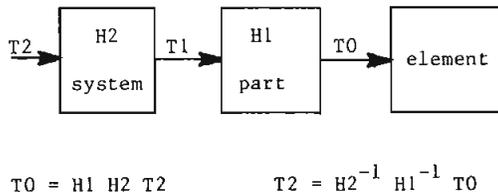
Figure 2: Filter Representation of a Test
