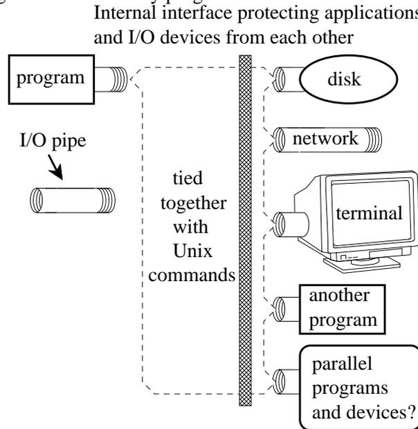
FIG. 3: Data pipes in Unix
