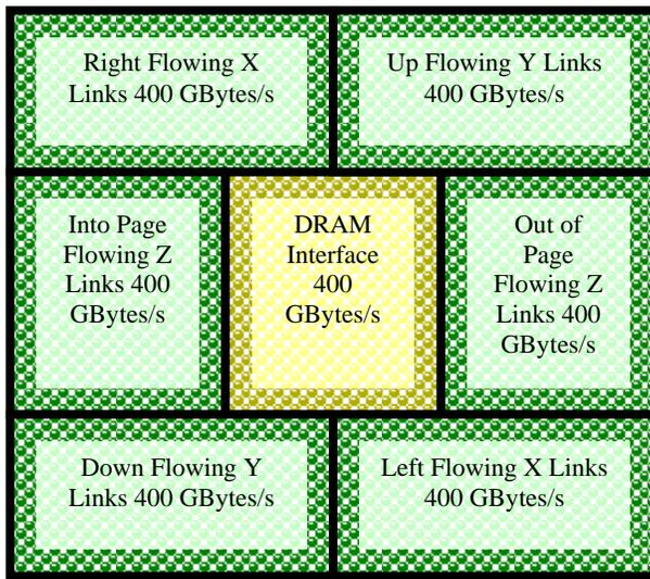
Figure 3: Example Layout of Interconnect Across the Chip
