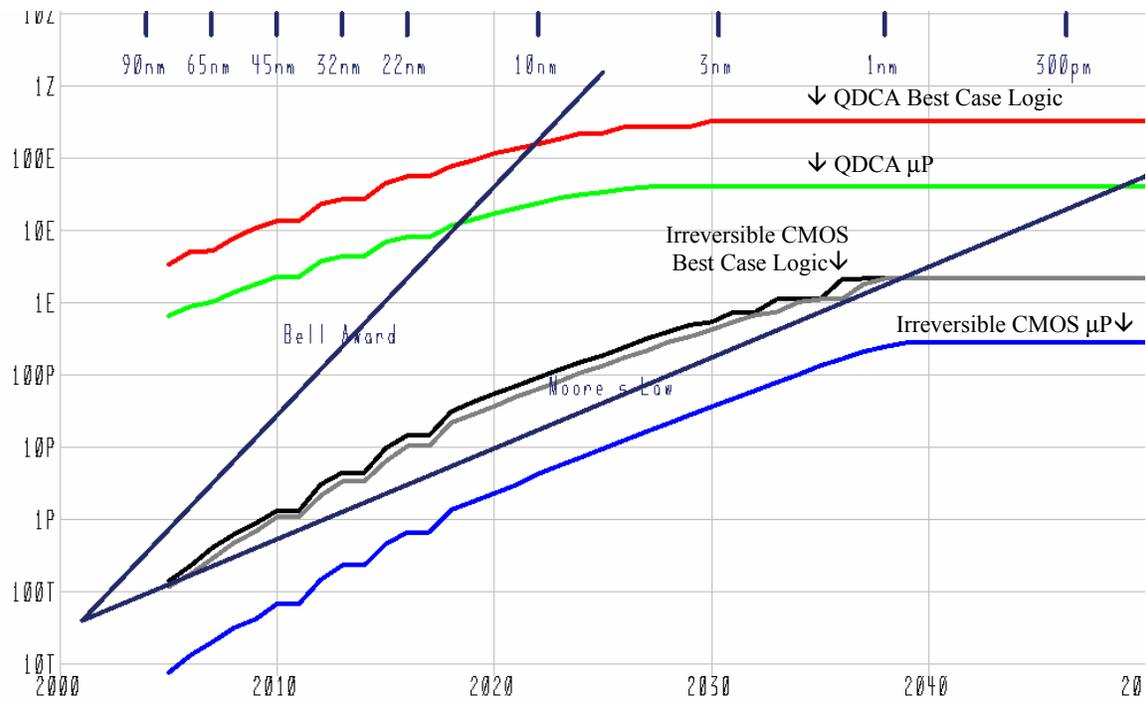
**Figure 7: Time Trend of various technologies for performing global climate modeling per [15]. Red=Quantum Dot Cellular Automata [22] with reversible logic and special purpose (non- $\mu$ P architecture); Green=Quantum Dot Cellular Automata [22] with reversible logic and  $\mu$ P parameters; Black=irreversible CMOS with special purpose (non  $\mu$ P) architecture, Blue= irreversible CMOS  $\mu$ P.**
