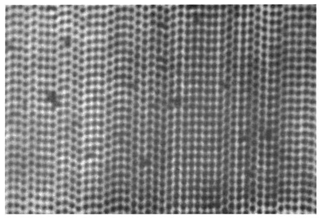
FIGURE 6 — EXPERIMENTAL DIGITAL AUDIO DISC
