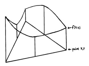
Figure 1: A Triangular Finite Element
